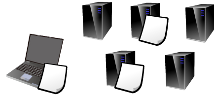
Fig. 2: GlusterFS places replications on servers.
